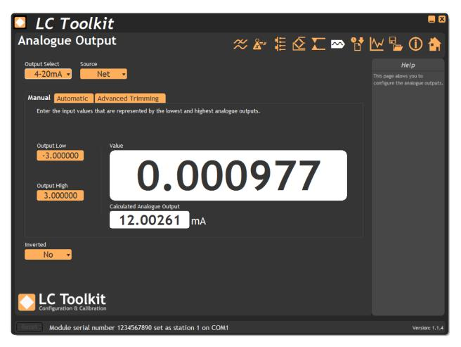
**Output Select** – Choose between 4-20mA current output or 0-10V voltage output.
