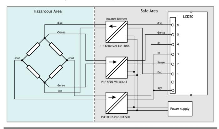
Because the barriers are fully isolated, the **REF** connection <u>MUST</u> be made to ensure that the LCD20 input stage is biased correctly.
