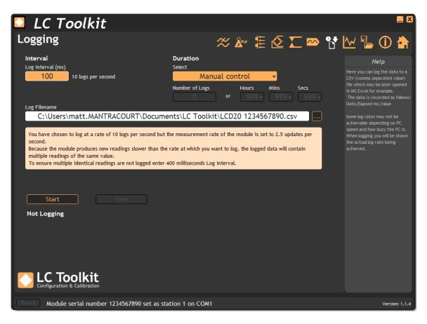
Once the logging starts the actual achieved log rate will be displayed at the bottom of the window. This is useful for diagnostics such as when a heavily burdened PC is slowing the log rate.
